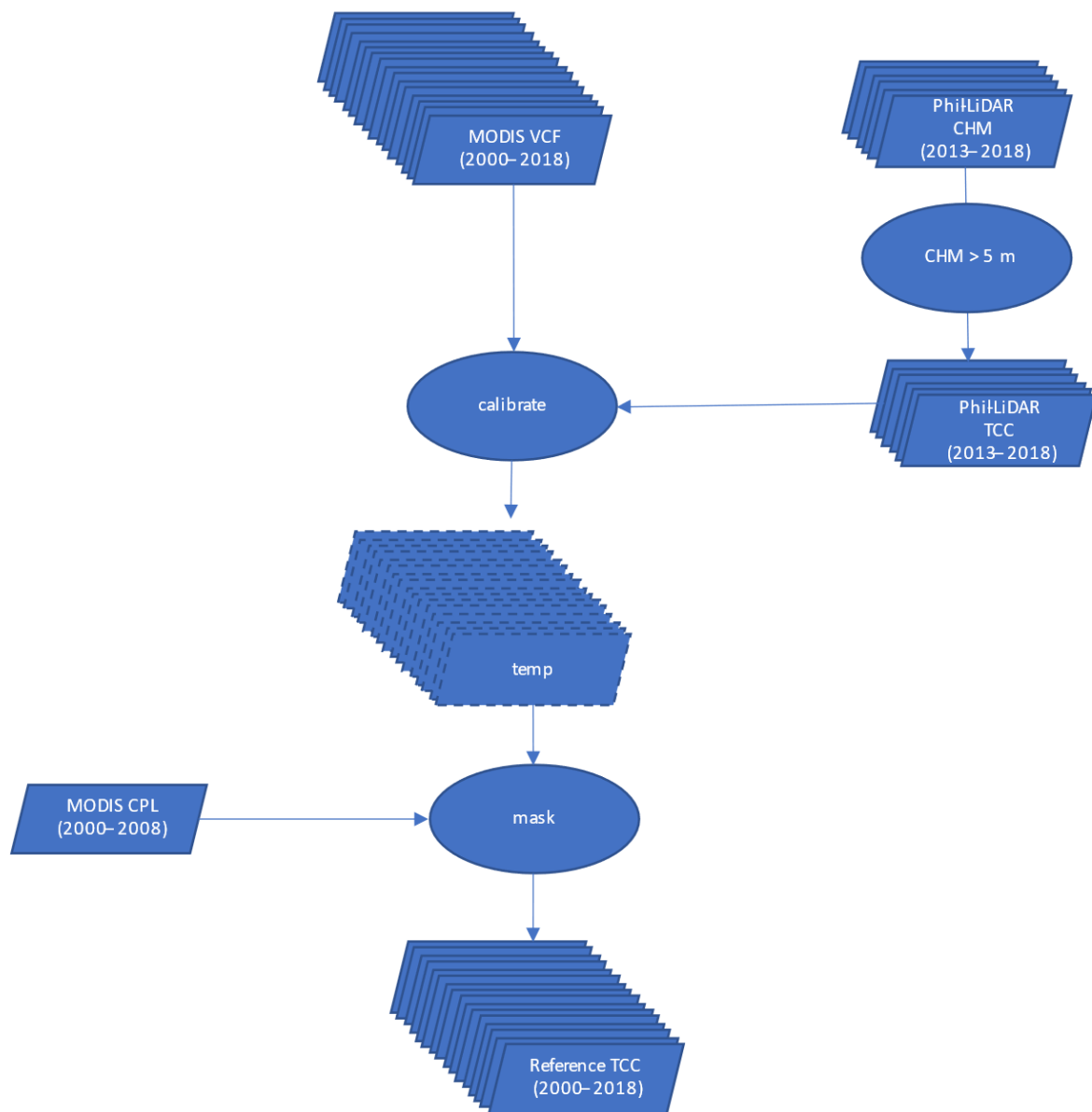
Figure 4. Calibration of MODIS Vegetation Continuous Fields (VCF) Tree Canopy Layer to Phil-LiDAR Canopy Height Model (CHM) and subsequent masking based on MODIS Cropland Probability Layer (CPL) to produce reference estimates of tree-canopy cover. The calibration model is fit to a training sample from the years 2013 to 2018 and applied to the 2000 to 2018 population from which the sample was drawn.
