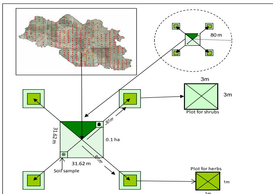
**Fig 4: Layout of the sample plot in plain**
