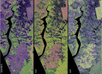
Synergistic use of satellite sensors can help to achieve the confidence required for operational monitoring. These three synthetic aperture radar images of Central Kalimantan, in the Indonesian part of Borneo, were acquired by ALOS PALSAR (left) ASAR on Envisat (middle) and TerraSAR-X (right). © 1AXA-METT/ESA/DLR
