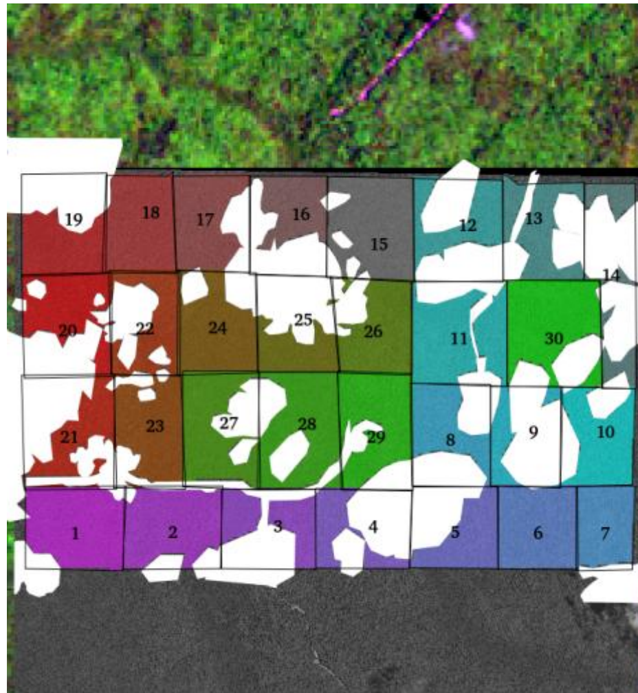
Figure 12: Concession study area with recent logging divided into 30 analysis regions. White areas represent clouds, cloud shadow and direct infrastructure (e.g. roads). These areas were omitted from the analysis.
