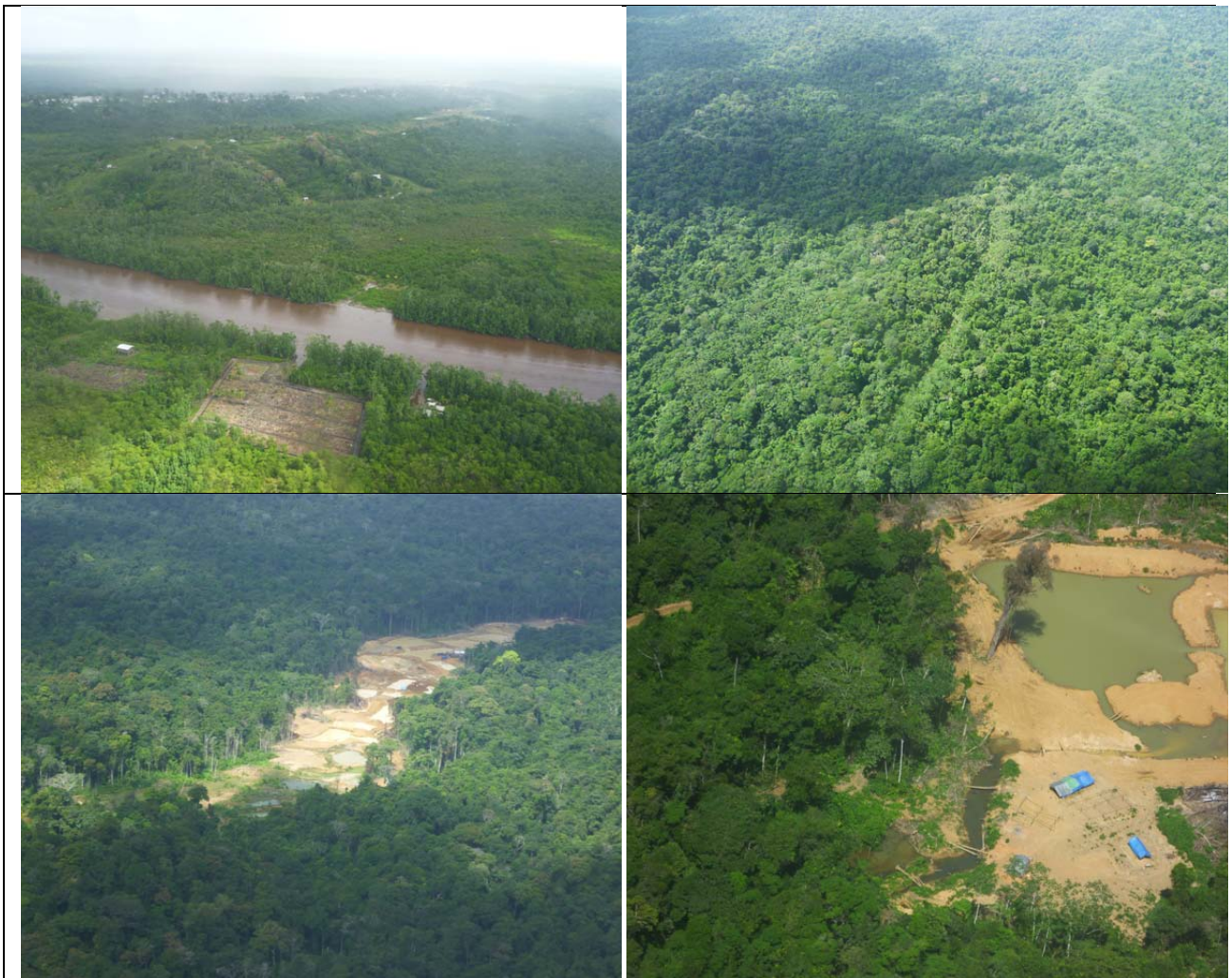
Figure 3-4: Example over flight photography (TL: clearance for agriculture; TR secondary road almost invisible; BL mining; BR zoom of mining camp / dredge)
