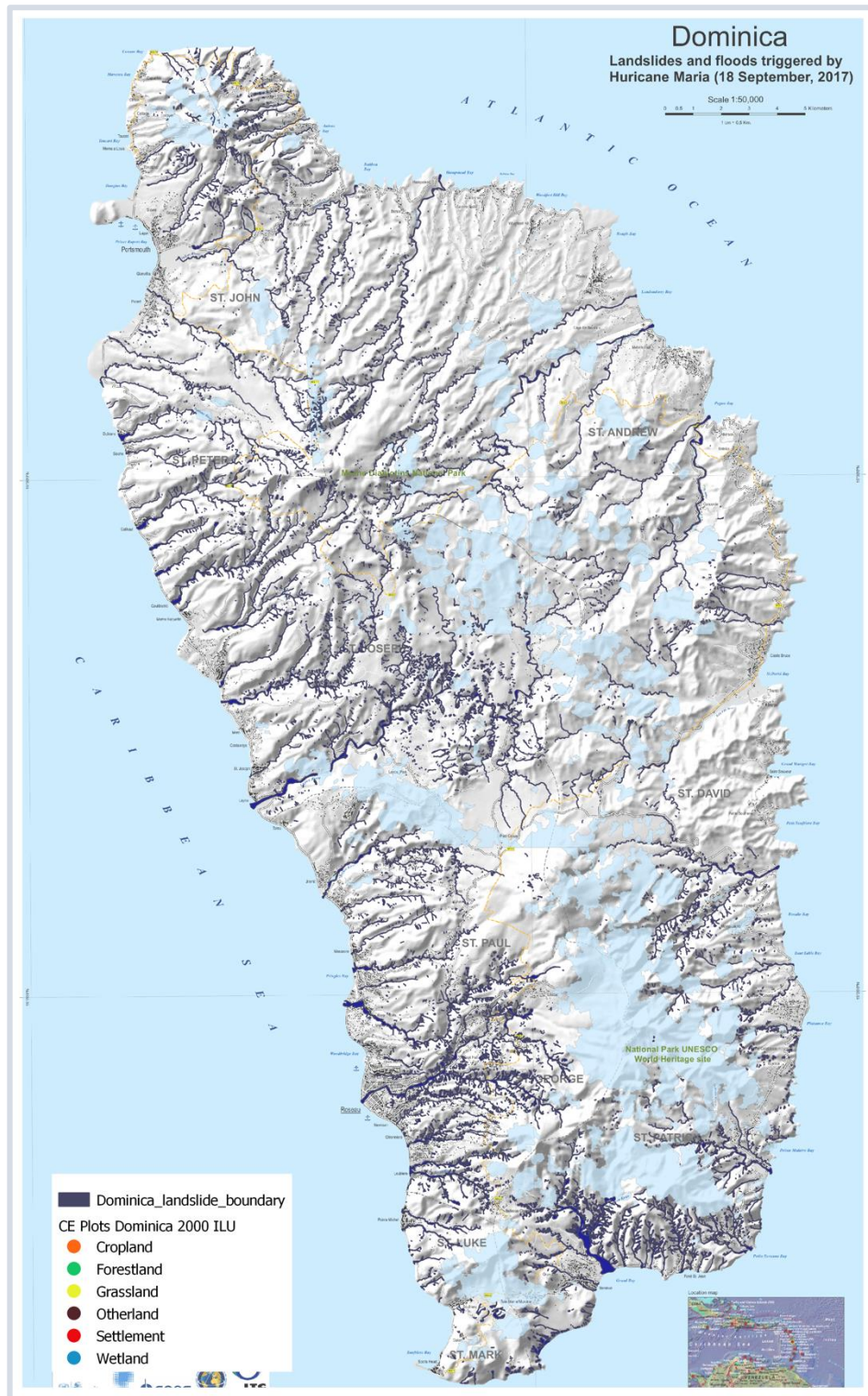
Figure 24 Landslides assessment after hurricane Maria (2017)
